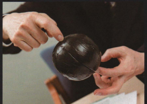
This is the specimen, a module wrapped in rubber like a baseball. The key to solving the problem is to use point contact.
