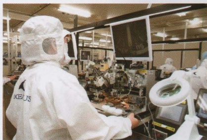
The G-shaped worktables are the Premium Production Line, and only those excellent technicians selected from different production procedures are permitted to enter this sacred place. The main tasks on these tables are the installation of minute/hour hands and dials, and the vertical and horizontal fine tuning. These technicians are all female, capable of long-time standard operation. 350~400 watches are produced here per day.
