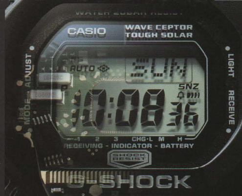
GW-5600 was created in 2005 by mounting the Tough Solar power system on the original square model. The limited dial size of this model delayed the use of this new technology, which requires reduced antenna size and improved sensitivity for radio wave reception. Meanwhile, the Tough Solar technology requires smaller LCD for power conservation.
